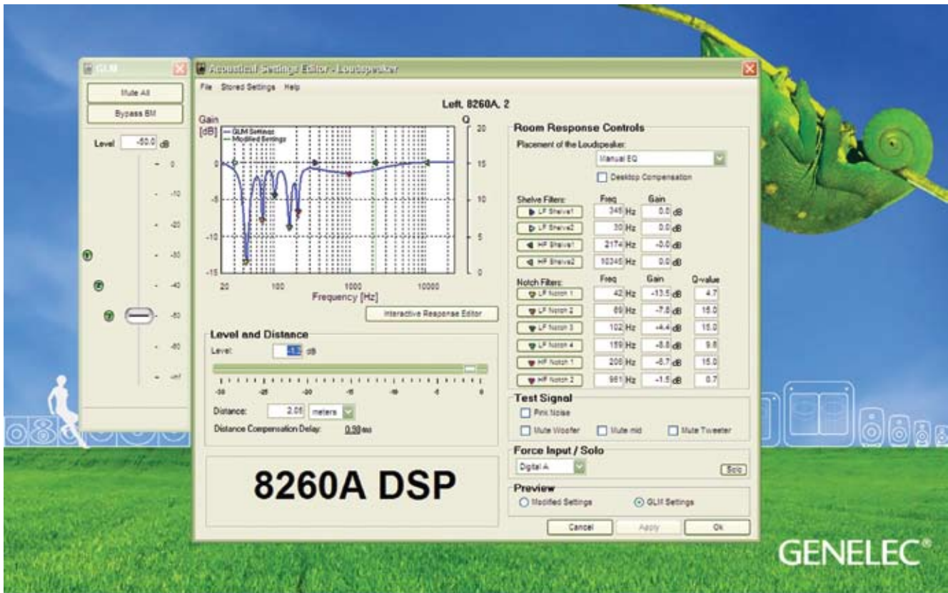
Figure 9: GLM Acoustical Settings Editor Window for 8260A with the GLM Volume fader on the left.
